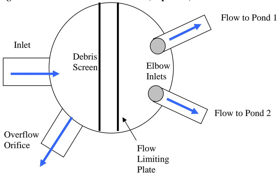
Inside each distribution structure, two plastic plates have been installed. The plate closest to the inlet is the debris screen. This plate has been perforated with numerous 1” diameter holes. This plate will catch sticks, leaves, or other debris that enters the distribution structure. The debris screen can be lifted out of the box for cleaning when necessary.
