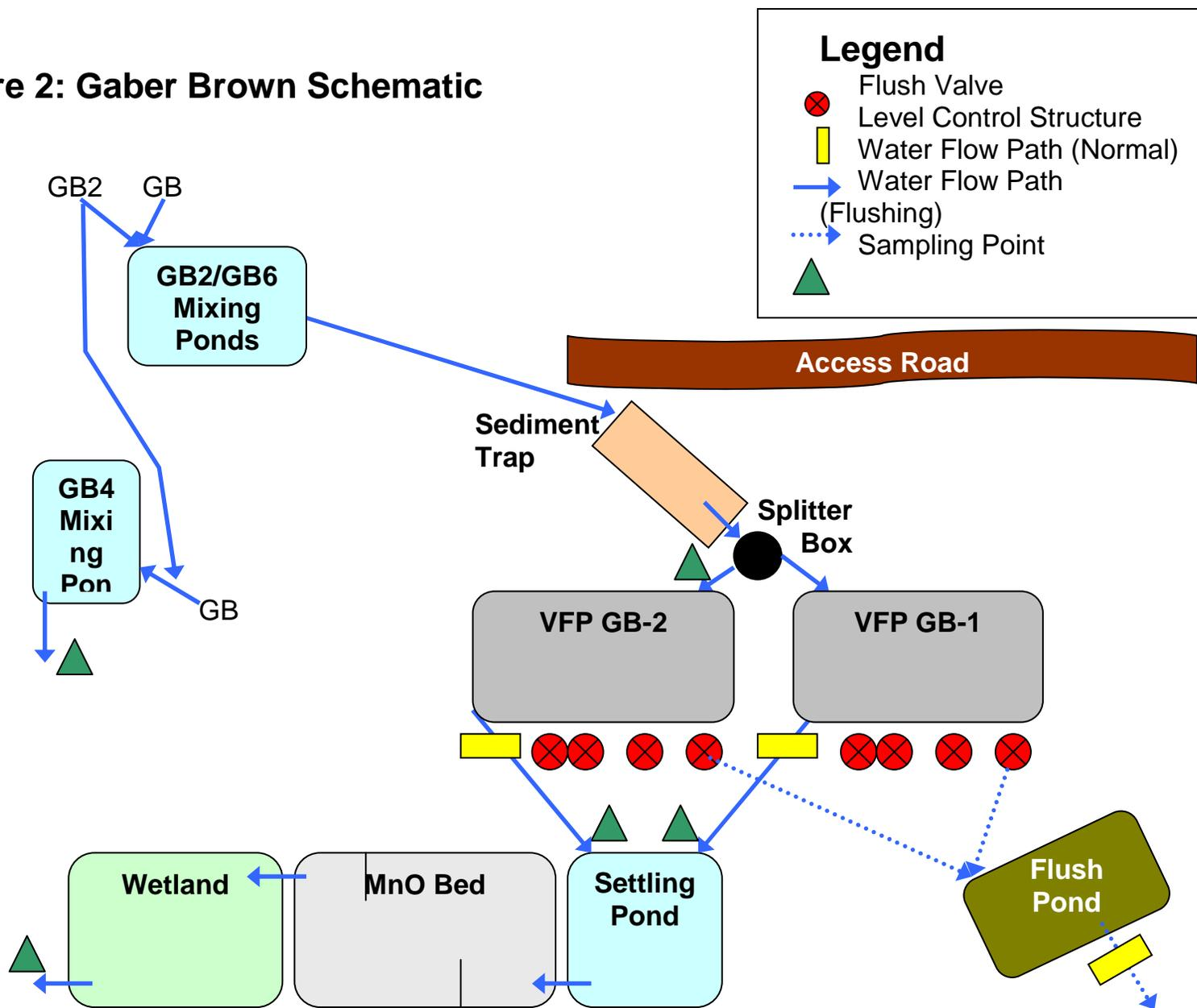
small ponds. This mixing allows the aluminum to form a solid and settle in the ponds. About 4 gpm of water from GB2 is required. This amount is adjusted via a valve at the GB4 pond location. The pipeline should be cleaned out every month by opening the valve and allowing it to flush until the water is clear (5-10 minutes).
